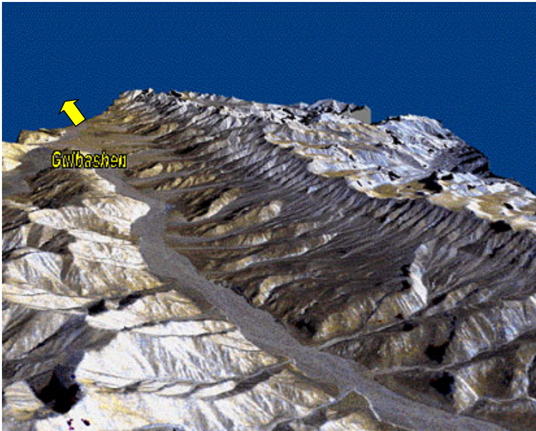
Three-dimensional perspective of the Karakax valley created by combining two spaceborne radar images using a technique known as interferometry. The image was acquired by the space shuttle Endeavour in October 1994. The image center is at 36^{\circ}10' North and 79^{\circ}20' East, looking westwards with Kun Lun chain to the right with peaks at over 6000m. The sloping line somewhat parallel the top of the chain is the Altyn Tagh fault. The position in the valley corresponds to a place approximately 15km East of Sumgal. The jade quarries at Gulbashan are approximately 70 kilometers downstream from this site. (Courtesy NASA Jet Propulsion Laboratory Pasadena USA)
